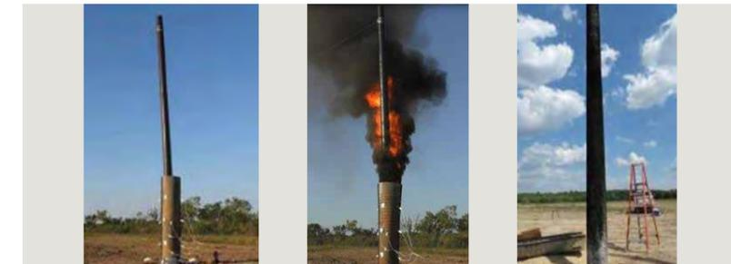
Pre-test (left), mid test (centre) and post test (right) wildfire testing of a Valmont utility pole
