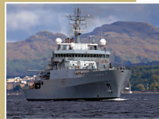
HMS Echo, one of two new multi-role Hydrographic/Oceanographic Survey Vessels. These are extremely capable vessels and are able to collect a wide range of hydrographic and oceanographic data, both on and off the continental shelf, using state of the art equipment.
